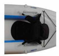
For the rearward seat, clip the back straps to the spray skirt D-rings and the foward straps to the D-rings just in front of the seat.
