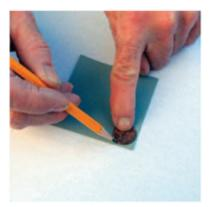
Trace the outline of a penny on the patch material and cut using scissors. Trace the outline of the penny on the boat. Coat the patch and boat with the repair kit glue.
